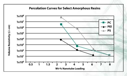
one nanotube to another, the higher the crystalline structure of a resin, the lower the volume of nanotubes required to complete the conductive array.
