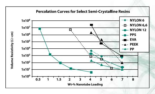
nanotube to another, the higher the crystalline structure of a resin (as in polyphenylene sulfide (PPS)), the lower the volume of nanotubes required to complete the conductive array.
